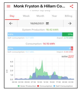
As the days grew warmer, we started the process of systematically turning off items which were the potential causes of the energy consumption spikes. In the end an immersion heater switch linked to a pump was causing the spikes. One flick of this switch and the mystery was resolved and our power consumption dropped immediately.
